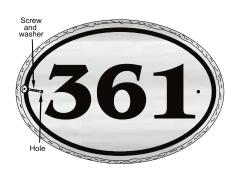
Step 3- Hand tighten screw while holding sign flush with surface. **Do not over tighten.** Over tightening can result in damage to the slate and siding.
